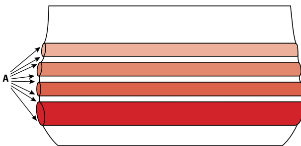
MULTI-PASS BOILER UNDER THERMAL STRESS
